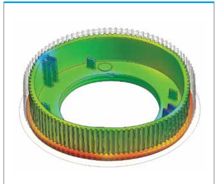
Figure 3 | Warpage prediction for a thermoplastic gear (magnified scale).
