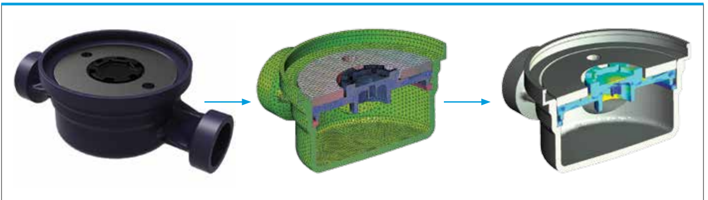
Figure 4 | Structural analysis of a water meter diaphragm made of glass-fiber-reinforced Radilon® PA6.12, from load and constraint definition to tension state prediction.
