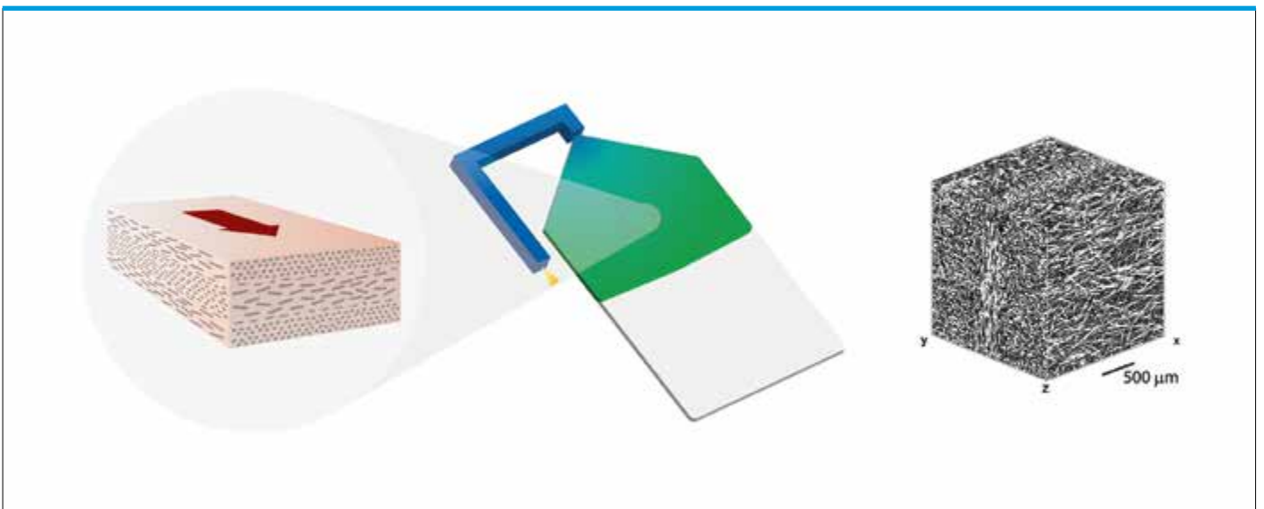
Figure 5 | Glass-fiber orientation in a part depends on how the cavity is filled during molding. A shell-core structure is typically obtained when thin plates are injection molded, as can be seen in the microtomographic scan image on the right.
