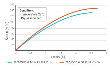
Figure 8: Stress-strain curve
