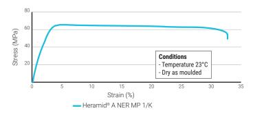
Figure 9: Stress-strain curve
